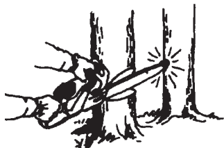
KICK GUARD® ALLOWS SAFE CUTTING NEAR OTHER TREES
